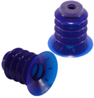
VGB4-XP35P-PU-Flex (DUO) 410.035.210.13 Ø 35 mm, HF = 11,6 N, veerweg = 22,0 mm, PU-Flex (DUO), 30-55° shore A (licht/donker blauw)
